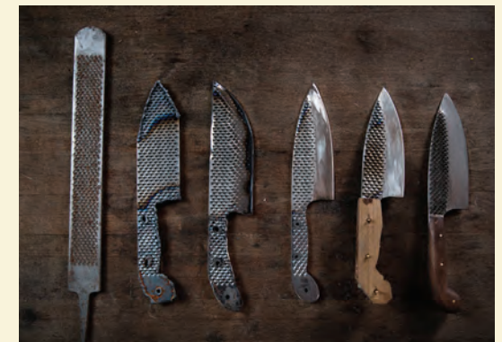
^ Showing the stages of the knife making, horse shoe rasp, cutting out with plasma cutter, forge, grinder, sander, wood handle and waxing, ships to its forever home.
