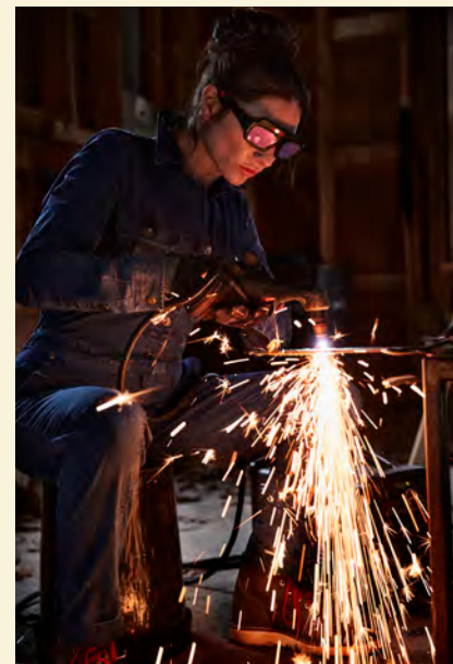
^ Showing the stages of the knife making, horse shoe rasp, cutting out with plasma cutter, forge, grinder, sander, wood handle and waxing, ships to its forever home.
